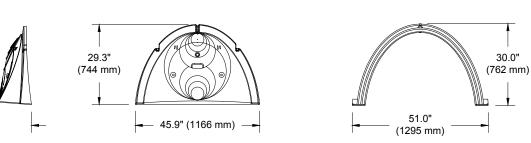
51.0" X 30.0" X 85.4" (1295 mm X 762 mm X 2169 mm) SIZE (W X H X INSTALLED LENGTH) CHAMBER STORAGE 45.9 CUBIC FEET (1.30 m<sup>3</sup>) 74.9 CUBIC FEET MINIMUM INSTALLED STORAGE (2.12 m<sup>3</sup>) WEIGHT 75.0 lbs. \*ASSUMES 6" (152 mm) STONE ABOVE, BELOW, AND BETWEEN CHAMBERS
