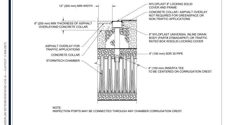
4" PVC INSPECTION PORT DETAIL (SC SERIES CHAMBER)
